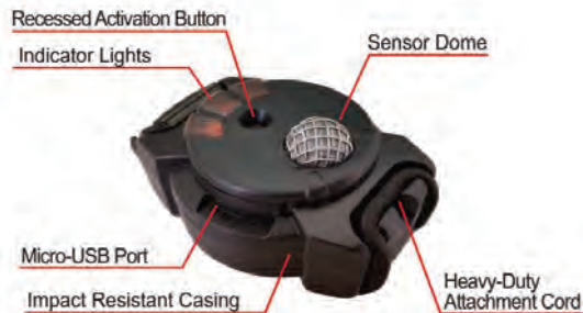
Figure 6 ("BlackBox Biometrics, the Blast Gauge(R) System, Gen. 7"
