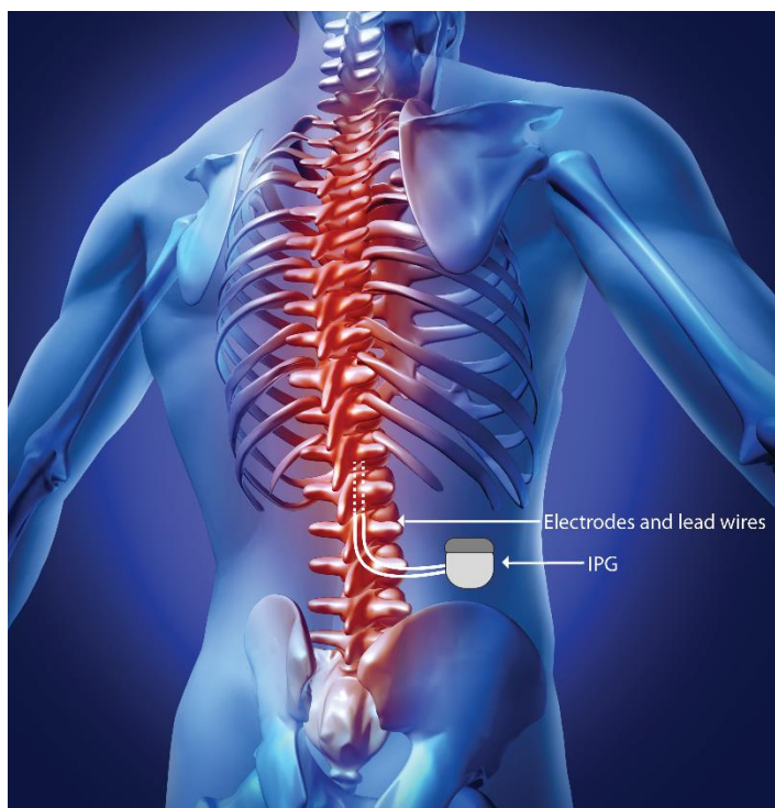
Figure 1. Illustration of spinal cord stimulation (SCS) system with implantable pulse generator (IPG) and electrodes placed between the spinal cord and vertebrae (epidural space)
